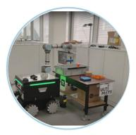
The scenario consisted of a table and a box where the objects were placed. A marker was positioned on one side of the table to help the robot move to a point close to the table and access all the objects in the box. Another marker was placed in a corner of the table to assist the algorithm in calculating the object's position in the world, enabling the robot to locate the objects from its posi-
