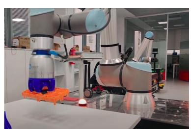
ROS+, the mobile manipulator robot that will execute advanced AI algorithms to detect and identify the components on the workbench, compute the order to pick the components and where to place them, find the best bile Robots) and manipulation of robotic arms are grasping pose and calculate and follow the arm trajecto-
