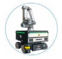
A mobile manipulator robot like RB-KAIROS+, the one involved in ULTIMATE, allows the arm's functions to be expanded, thus improving operational capacity and increasing return on investment.
